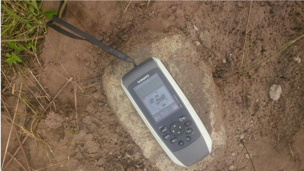
Figure 2: A Hand held GPS on a Cadastral Survey Beacon.
