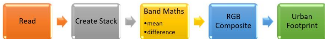
Figure 9 – Workflow - obtaining the urban footprint – main steps
