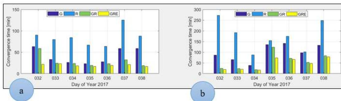
Figure 2: Average convergence time for standard dual-frequency PPP (a) and ionosphere-constrained dual-frequency PPP (b) per day.
