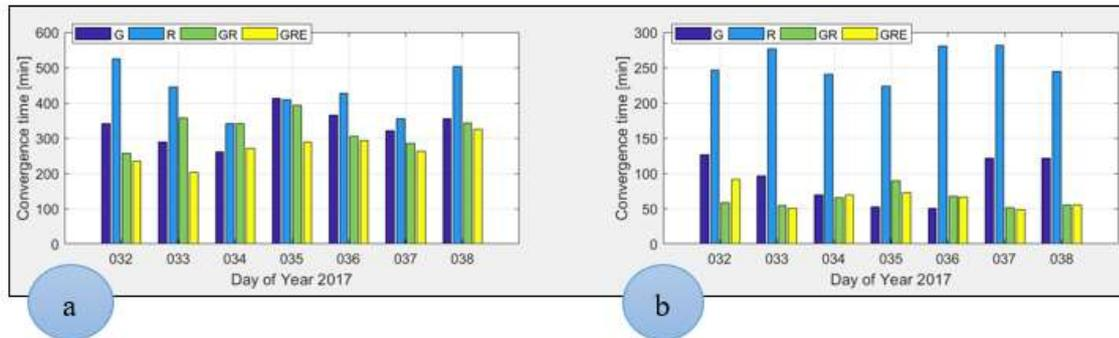
Figure 1: Average convergence time for standard single-frequency PPP (a) and ionosphere-constrained single-frequency PPP (b) per day.
