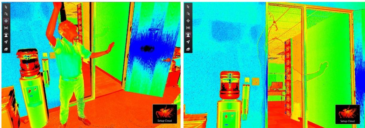
Figure 13a and 13b: Effect of the moving object filter in Cyclone REGISTER 360.
