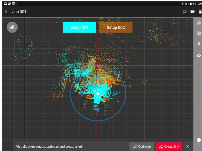
Figure 10: Visual alignment in Cyclone FIELD 360.
