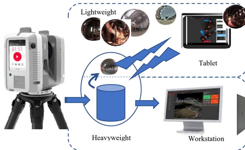
Figure 9: Data transmission and synchronisation between the three components of the RTC360 solution.
