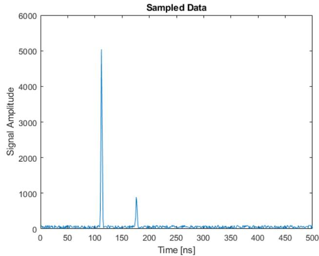
Figure 4: Emitted EDM pulses on RTC360.
