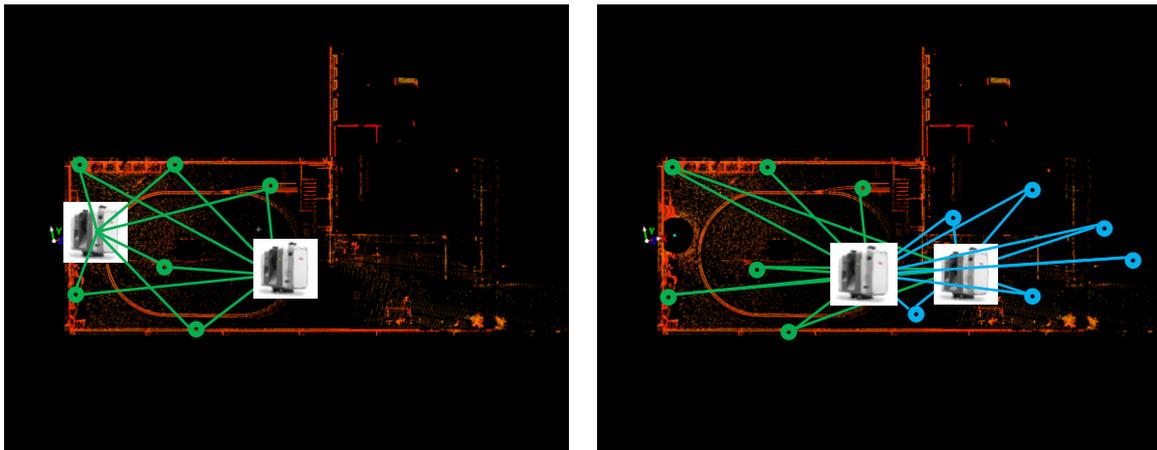
Figures 8a and 8b: 3D features resection and forward intersection.
