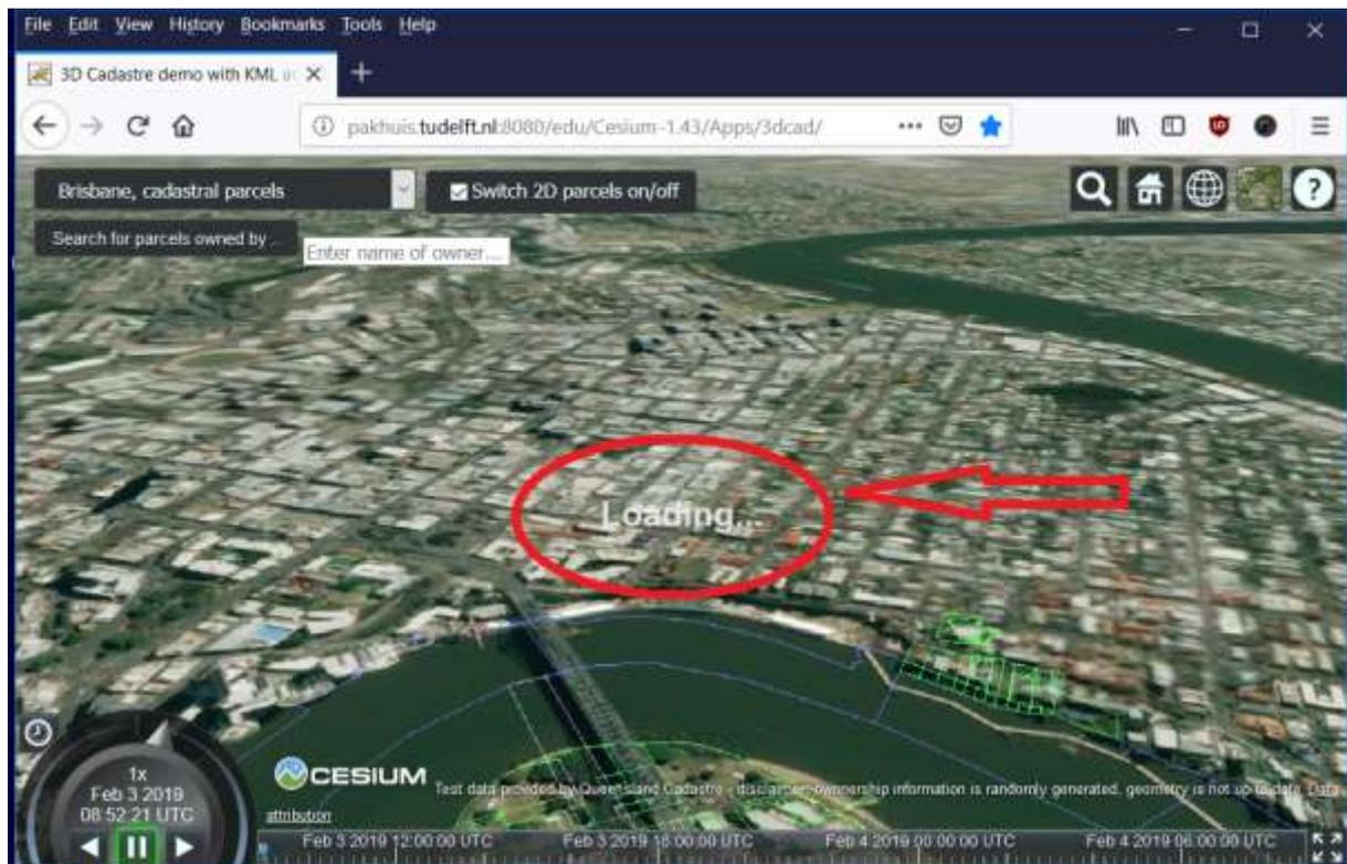
**Figure 4. Showing a feedback message during the loading of data, which takes some time. Note that the message “Loading...” (red oval and arrow added to this image) is actually blinking, giving the users the impression of ongoing activity.**
