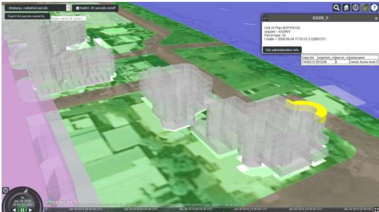
**Figure 1. Web-based 3D cadastral client showing the selection of an apartment (yellow highlight, on the left side of the image)**
