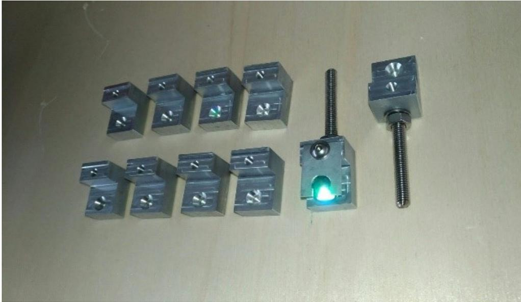
*Figure 5: Special holder for the LT reflectors in different manufacturing steps*
