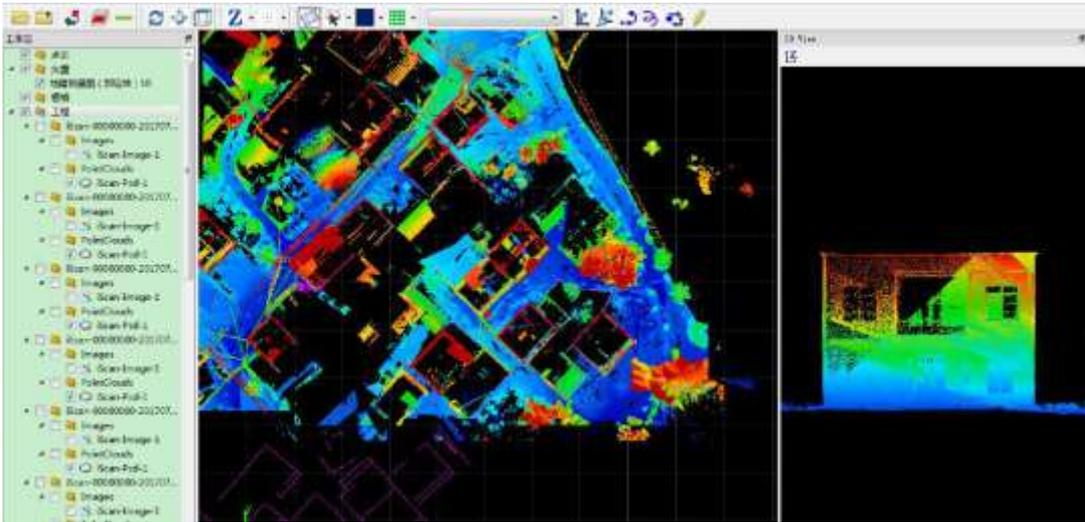
We design a specific software for cadastral drawing, the point cloud data can be used for generate cadastral data automatically.
