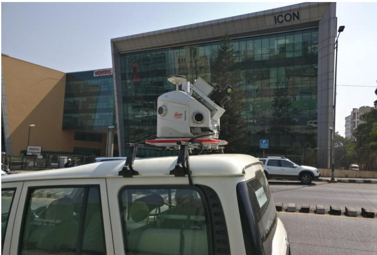
About 50 Km to 80 Km of city road network can be easily captured in a day using one unit of such mobile LiDAR system. Many solution providers are available in the industry viz, Trimble MX9, Leica Pegasus Two Ultimate, RIEGL VMX-2HA, Topcon IP-S3 HD1, Teledyne Optech's Maverick, HI-TARGET HiScan-C, with wide range of specification and price range to choose from.
