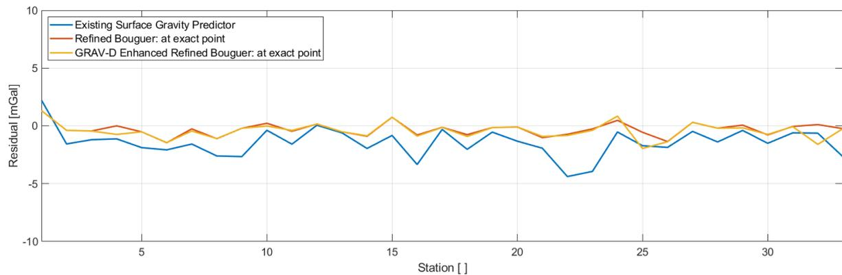
Figure 15: GRAV-D control station prediction residuals for prediction methods that rely on the existing surface gravity data
