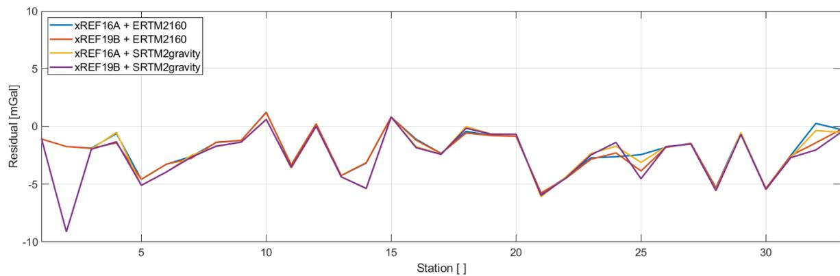
Figure 14: GRAV-D control station prediction residuals for variants of the reference model enhanced with terrain
