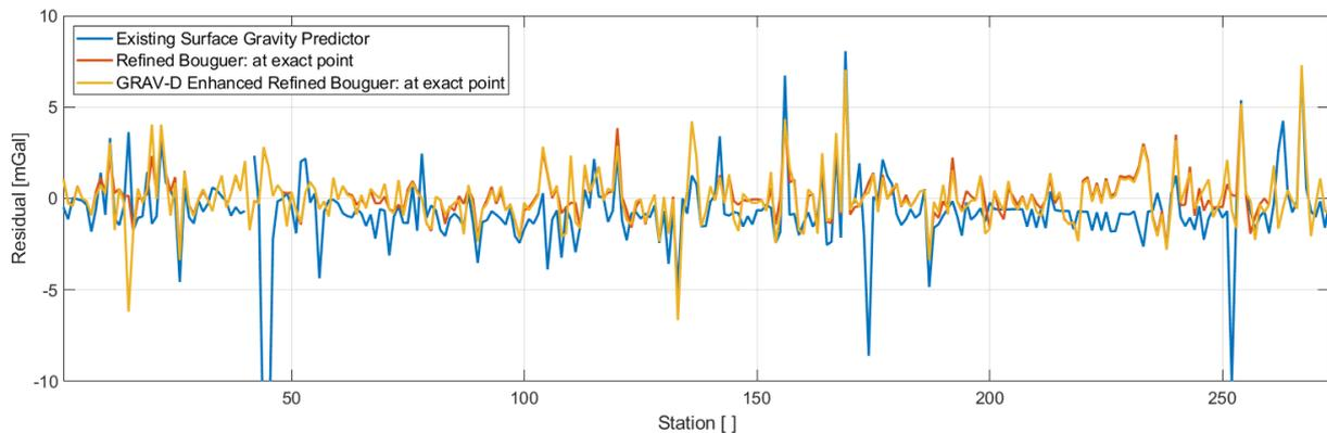
Figure 12: RELBASEA station prediction residuals for prediction methods that rely on the existing surface gravity data
