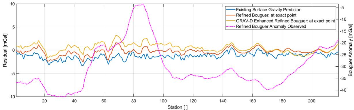
Figure 5: GSVS11 station prediction residuals for prediction methods that rely on the existing surface gravity data
