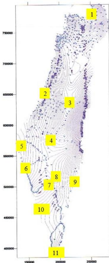
Fig. 3. Eleven locations (numbered squares) where the OGUM experiment was held in Israel, on a background of the SOI undulation map (contour line every 25cm) based on approximately 850 points (dots). The numbers denote the region, as appearing in Table 1.
