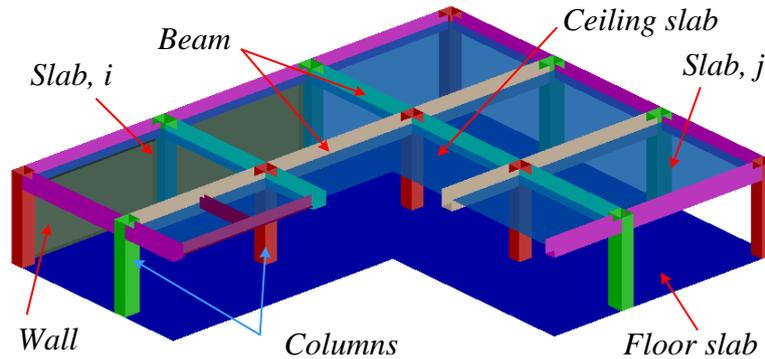
Figure 2. Structural elements in common reinforced concrete buildings
