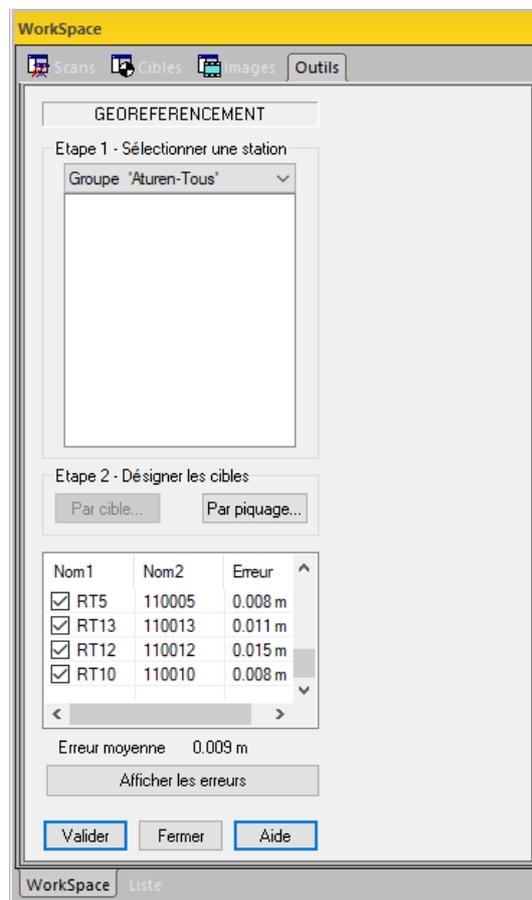
Fig. 8 Quality results from georeferencing of the point cloud
