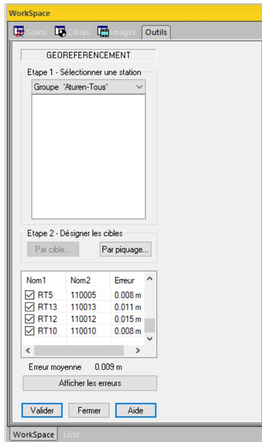
Fig. 8 Quality results from georeferencing of the point cloud
