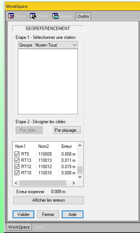
Fig. 3 Quality results from georeferencing of the point cloud
