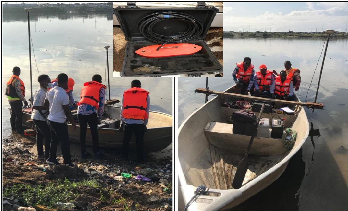
Figure 2. mobilizations and calibrations (left), the Kongsberg EA440SP echosounder used (top) and data collection (right)
