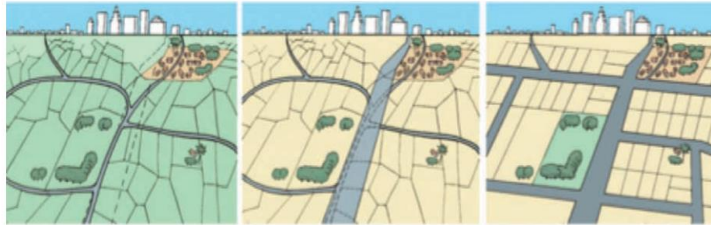
Before: Proposed Road Alignment After: Arterial Road Acquisition Inefficient and inequitable development After: With Land Readjustment Opportunity to plan, service, and finance development. All stakeholders benefit.
