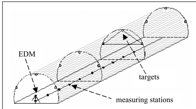
Figure 1: Arrangements of targets and of EDM measuring stations along the tunnel axis.
