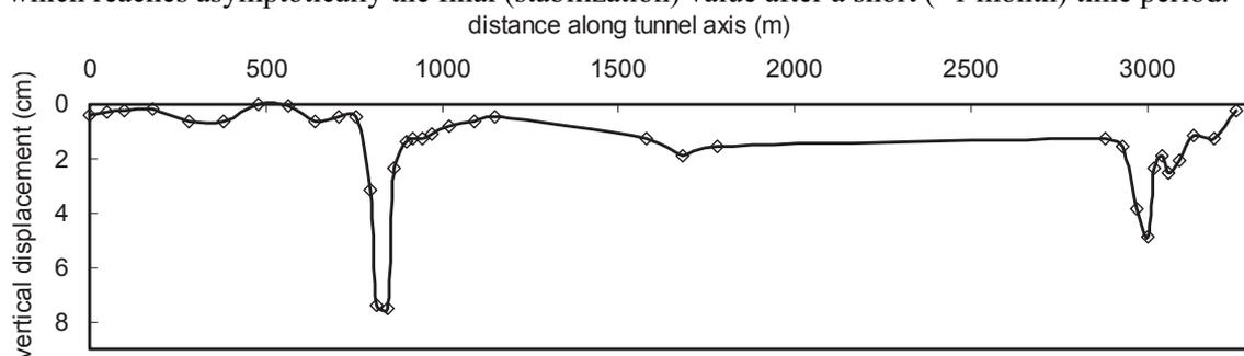
Figure 3: Local high convergence at points of high deformation affected adjacent tunnel segments as well, producing a swell-type deformation along a distance (data from Bolu tunnel, Turkey).
