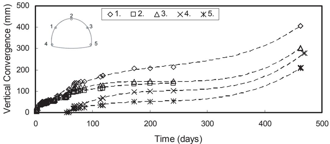
Figure 4: Resumed deformation after a stabilization period (between 170 and 240 days) for one section of the Kallidromo tunnel, Greece
