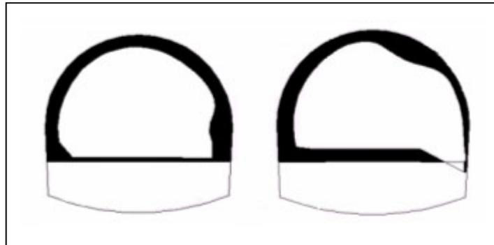
Figure 2: Representative deformed profiles from Tymfristos tunnel, Greece, a long time (1 year) after the excavation. Real scale convergence is indicated by black.
