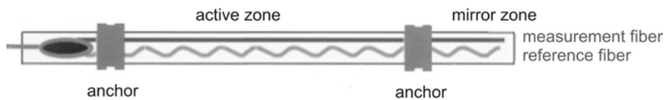
Fig. 5: Sensor of the SOFO System (after Inaudi and Vurpillot, 1999)
