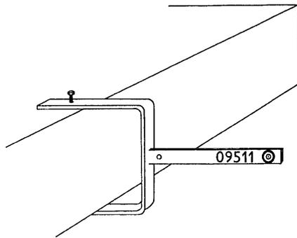
Fig.2 Sign for horizontal deformation measurement at Lafranconi Bridge in Bratislava
