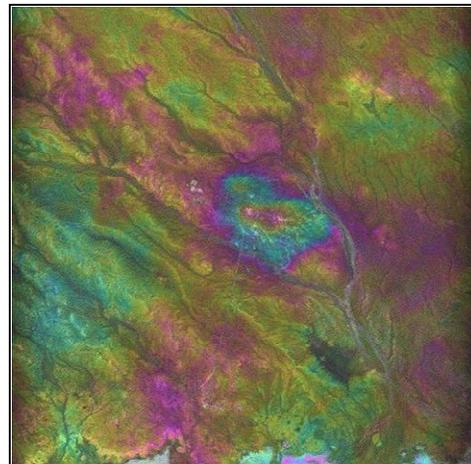
Figure 1 - Deformation mapped by InSAR at an oil field in Oman.
