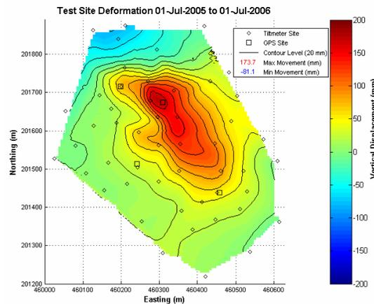
Figure 3 - Deformation calculation over one year from an integrated tiltmeter and GPS array.
