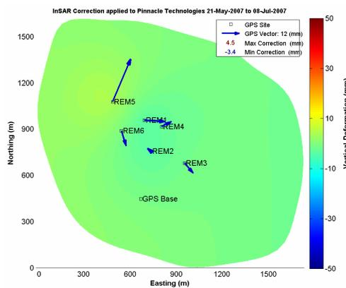
Figure 6 - Correction applied to InSAR image to match GPS in the line of sight
