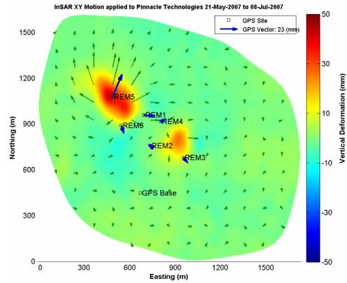
Figure 7 - Estimated Easting/Northing motion vector field
