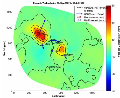
Figure 8 - Final integrated GPS and InSAR results
