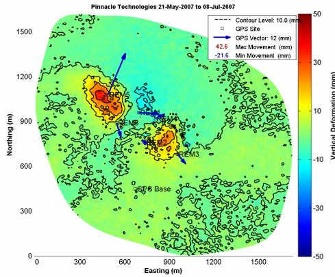
Figure 4 - Uncorrected InSAR deformation measurements from a test area.
