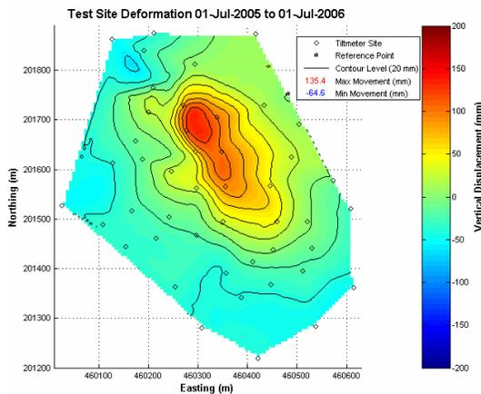
Figure 2 - Deformation calculation over one year from a tiltmeter array. GPS data was not used in the deformation calculations.
