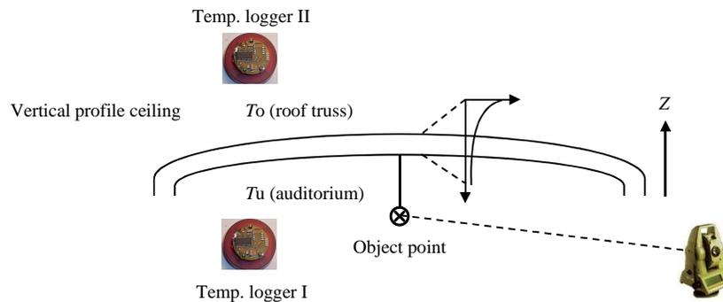
Figure 3 - Monitoring of thermal deformations.
