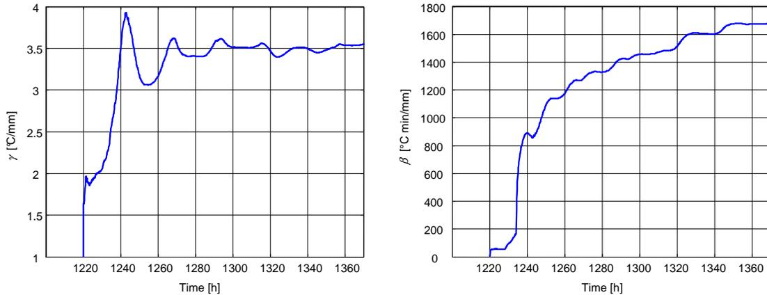
Figure 8 - Identification results for spring ( $\gamma$ ) and damping parameter ( $\beta$ ).
