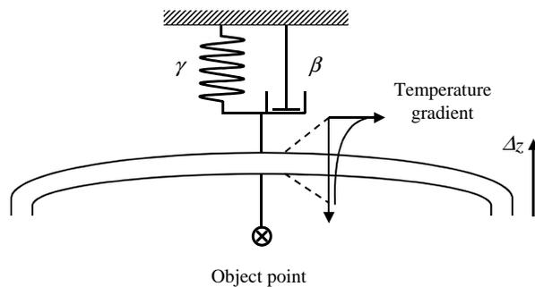
Figure 7 - Principle of the mechanical analogous model 'spring-damp-system'.
