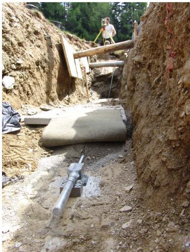
Figure 4 - Sensor S2 whilst embedding
