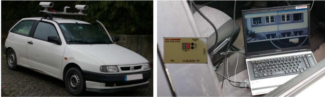
Figure 2 - Surveying vehicle and system components.
