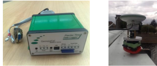
Figure 5a (left). A PTDL that was used for logging the tri-axial accelerometer data; 5b (right). An antenna set-up with a clasp on the bridge handrail.
