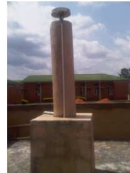
State of Osun CORS Antennae
