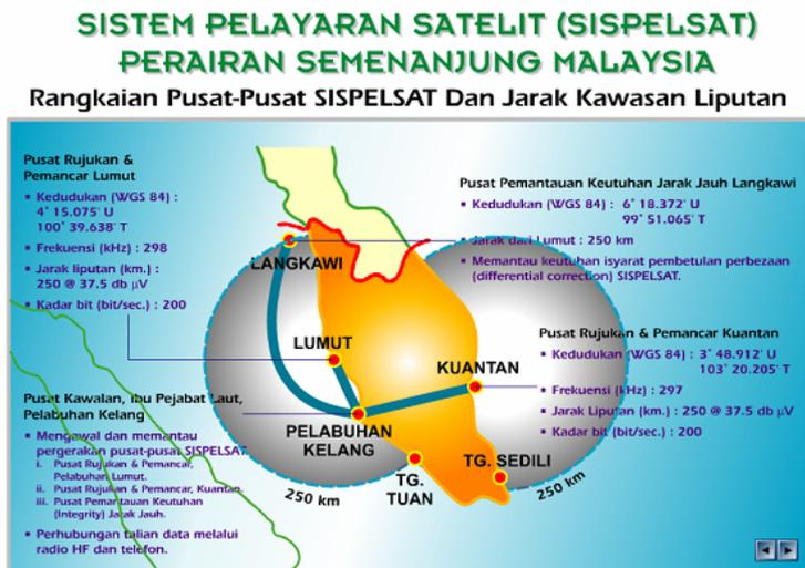
**Figure 1:** The Architecture of the SISPELSAT (source: Marine Department, 2004)
